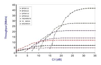
Figure 5 : Total system throughput over C/I with regard to PHY mode and ARQ
