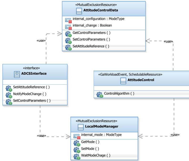
Figure 4: Class diagram of the ADCS component.
